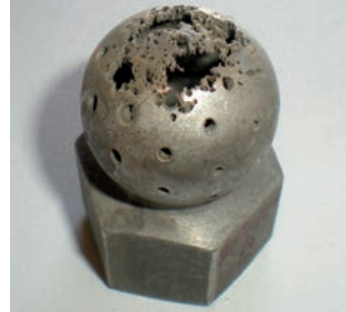
Fig. 1: Chemical corrosion of a spray ball
