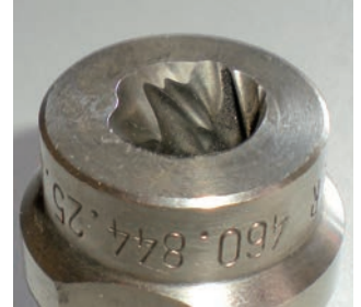
Fig. 2: Wear of a full cone nozzle
