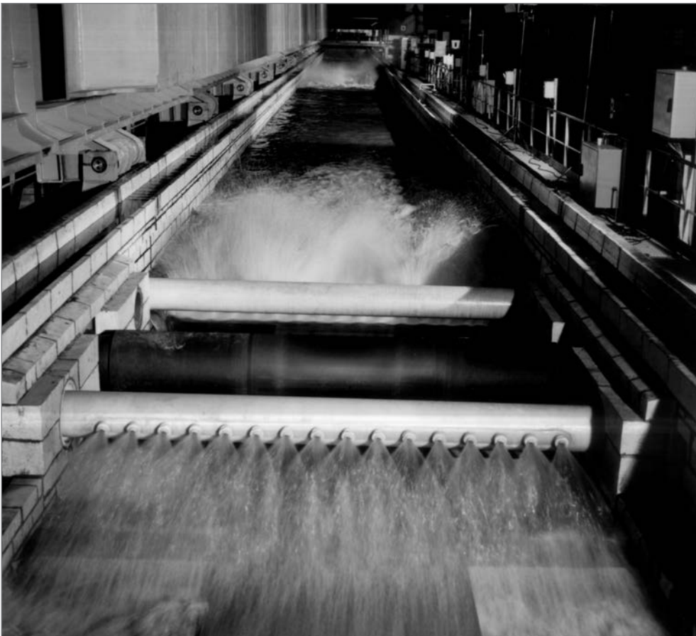
Pretreatment in a pickling line
