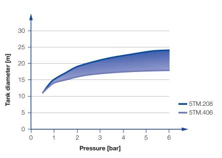
Overview of the tank diameter, depending upon the pressure of series 5TM
