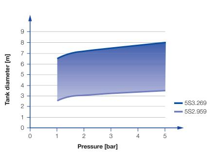
Overview of the tank diameter, depending upon the pressure of series 5S2 / 5S3
