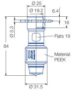
EHEDG-version Slip-on connection ASME-BPE 1997 (OD-Tube) 595.139.1Y.67 EHEDG-version Slip-on connection ASME - BPE 1997 (OD-Tube) 594.XX9.1Y.67
