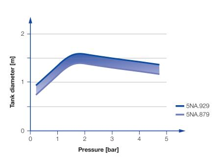
Overview of the tank diameter, depending upon the pressure of series 5NA
