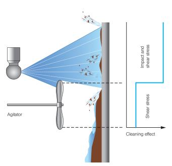
Figure 5: Cleaning mechanisms, impact and shear stress
