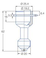
Slip-on connection ASME - BPE 1997 (OD-Tube)
