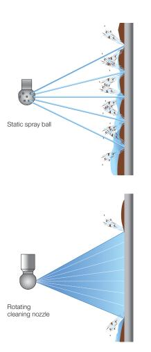
Figure 7: Comparison of rotating cleaning nozzles and static spray balls
