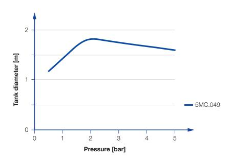
Overview of the tank diameter, depending upon the pressure of series 5MC
